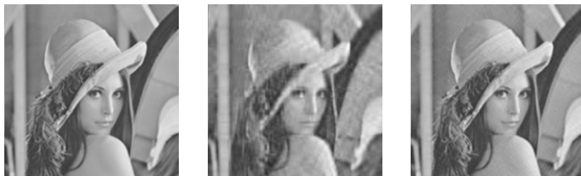
Figure 6.5. The original image ( left ) and those obtained using the first 20 ( center ) and 60 ( right ) singular values, respectively
