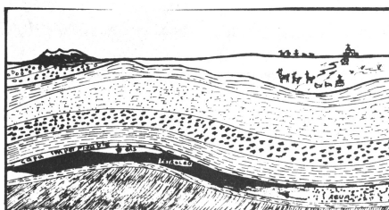
ANTICLINAL (trampa estructural)
