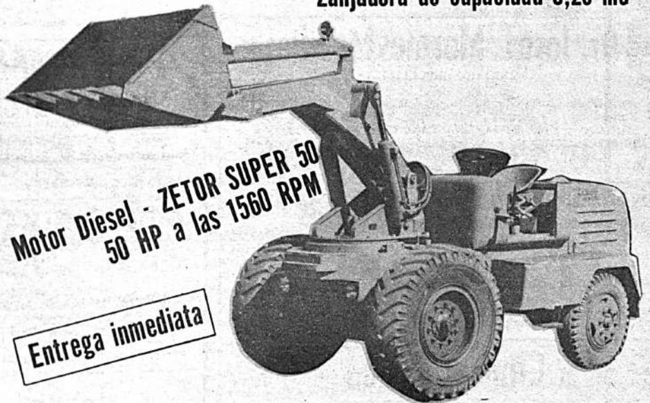
Motor Diesel - ZETOR SUPER 50
